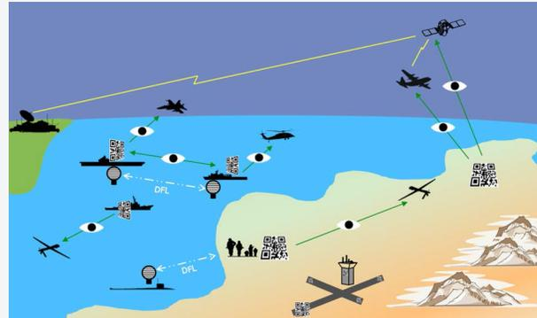
**Operational View (OV-1) shows line-of-sight (LOS) optical signaling via Quick Reaction (QR) codes and Digital Flashing Light (DFL). Only two radio frequency (RF) lightning bolts!**
